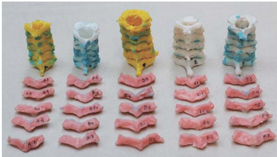
Fig. 7. Corresponding drill jigs for each of the three-dimensional–printed cadaveric spines.
