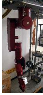
Fig. 13 The AMADEUS 7 d.o.f. manipulator used during the experimental trials.
