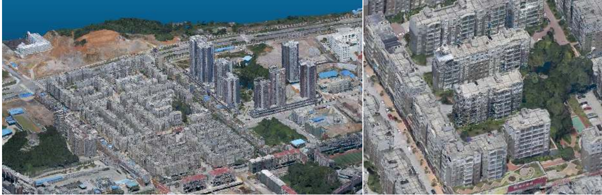
Figure 7: The point cloud reconstructions of a large area using RED-Net. The right is an enlarged part from the left scene.
