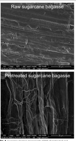
Fig. 4 Scanning electron micrographs (SEM) of pretreated and untreated sugarcane bagasse solid
