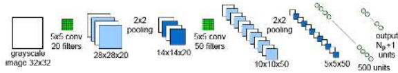
Figure 4. Architecture of \text{CNN}^{\text{part-det}} for part detection. The last layer outputs the likelihoods of the patch to correspond to each part or to the background.
