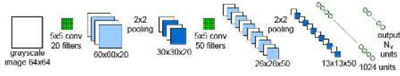
Figure 5. Architecture of a CNN \text{CNN}^{\text{cp-pred-}j} for predicting the projections of the control points.
