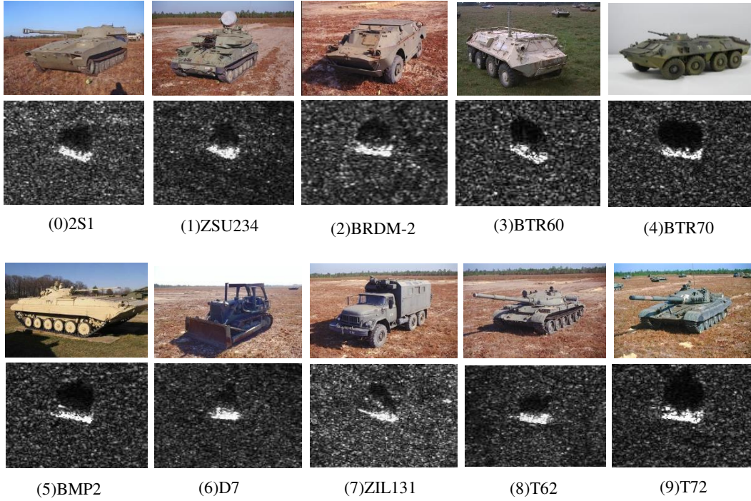
Figure 3: The SAR and optical images of ten types of targets in the MSTAR dataset.
