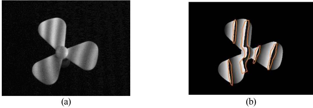
Figure 5. (a) Pattern with 5 fringes projected onto the blades of a propeller, and (b) relative phase map with discontinuities at fringe boundaries highlighted in orange.
