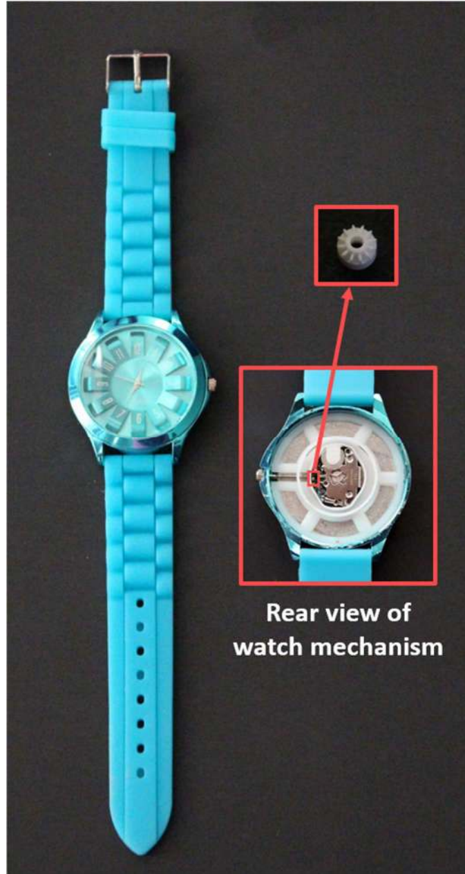
Figure 36. Wrist watch measured with micro-scale gear.
