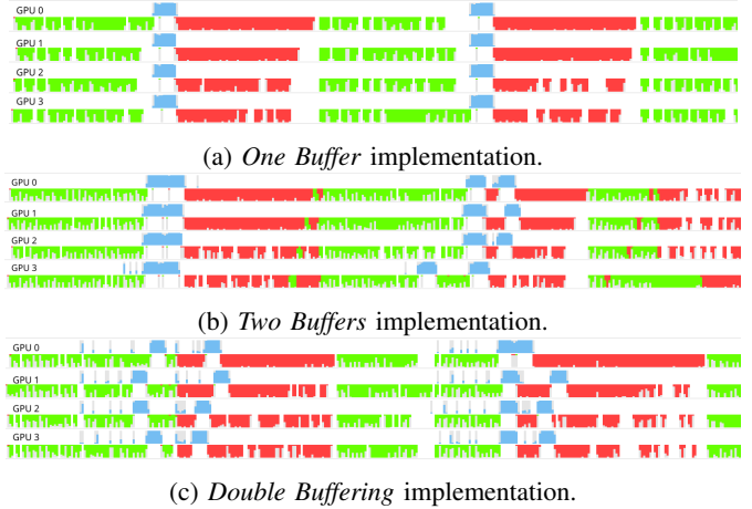
Fig. 3: 10 seconds of NVIDIA’s nsys traces showing memory transfers from host to four GPUs and vice-versa (in green and red) and kernel computations (in blue).
