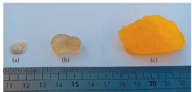
FIGURE 11: Image of dry TG powder (a), the swollen form of TG (b), and CMTG-GA (c).
