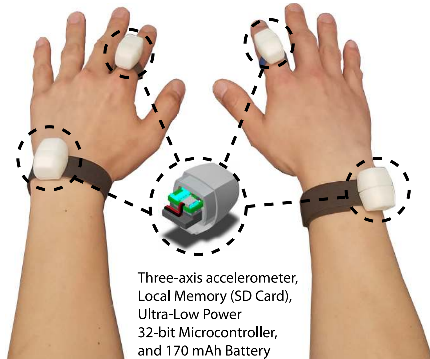
Fig 1. The miniaturized finger-worn and wrist-worn sensors used in the study. The sensor consists of a three-axis accelerometer enclosed in a waterproof case.
