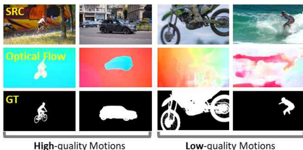
Fig. 2. Motion quality demonstrations, where the high-quality motions can usually separate salient objects from their non-salient surroundings nearby, while the low-quality motions cannot achieve this.
