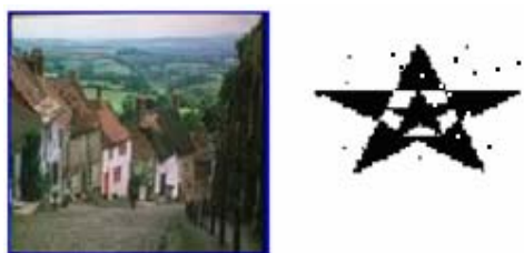
Fig. 6: Goldhill test image after hiding the watermark logo and the recovered logo at T=100.
