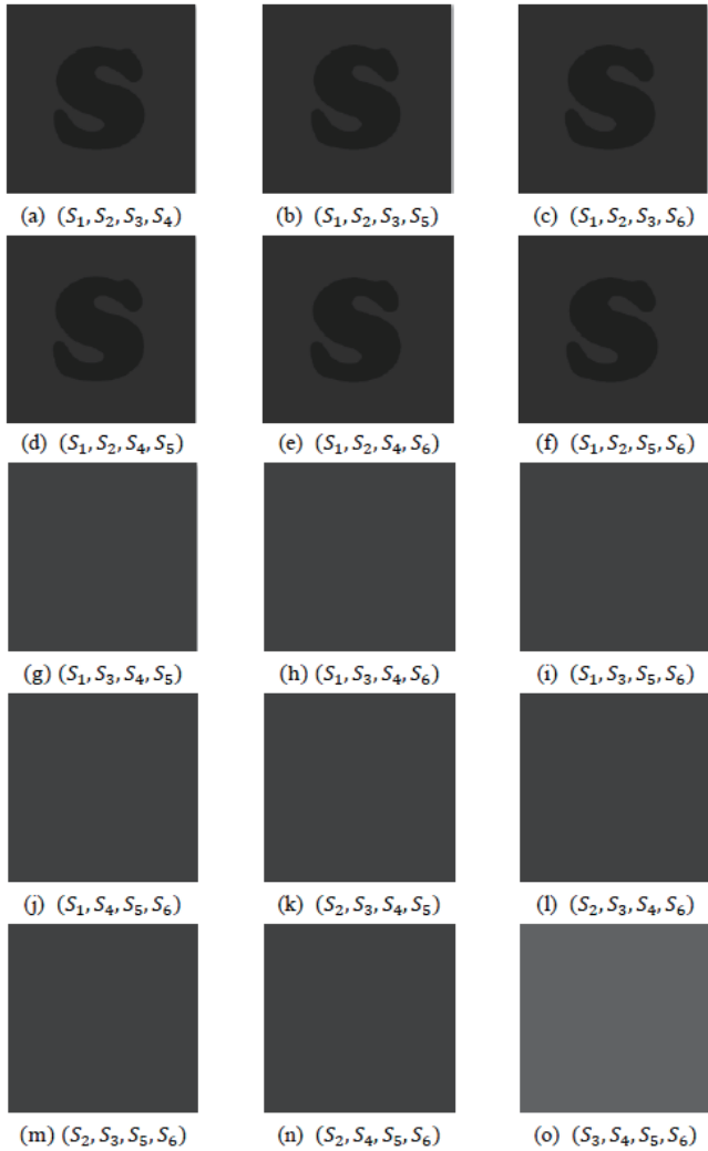
Figure 4: (a)-(f) the stacked results including two specific shares and two general ones; (g)-(o) the stacked noise-like results
