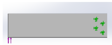
Figure 5. Finite element model of the cantilever structure.
