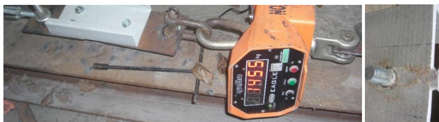
Figure 3. Experimental test of longitudinal shear strength.
