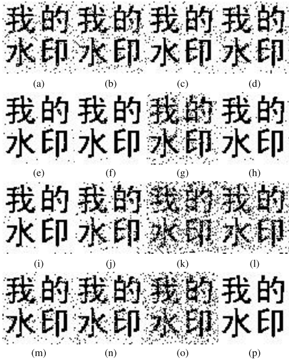
FIGURE 11. The extracted watermark image 1 for Lena image under different attacks: (a) Gaussian noise (0.05), (b) Gaussian noise (0.15), (c) Salt and Peppers noise(0.1), (d) Salt and Peppers noise (0.2), (e) Median filtering ( 5 \times 5 ), (f) Wiener filtering ( 5 \times 5 ), (g) JPEG compression(5%), (h) JPEG compression (20%), (i) Scaling (1/8), (j) Cropping (center 128 \times 128 ), (k) Cropping (Edge 64 \times 512 ), (l) Translation (5 pixels), (m) Rotation ( 5^\circ ), (n) Rotation ( 10^\circ ), (o) Rotation( 40^\circ ), (p) Rotation ( 90^\circ ).
