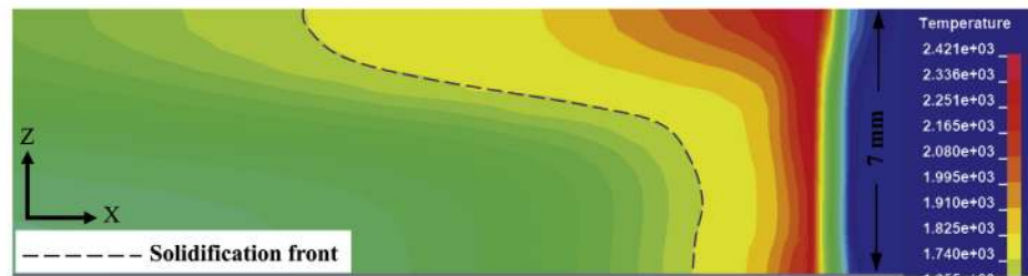
(c) Case III: full penetration: thin root ( P_l=7 kW, P_a=5 kW, v=2.5 m/min).
