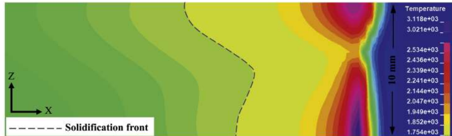
(b) Case II: full penetration: wide root ( P_l=12 kW, P_a=1.35 kW, v=0.9 m/min).
