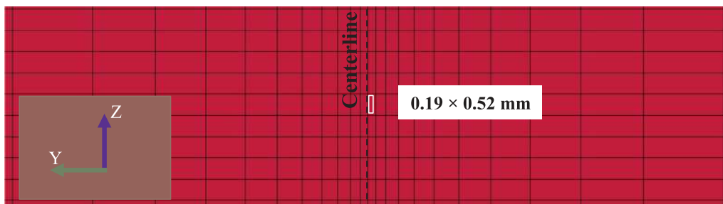
Fig. 12. Detail view of the mesh in the transverse cross section (refer to Fig. 11).
