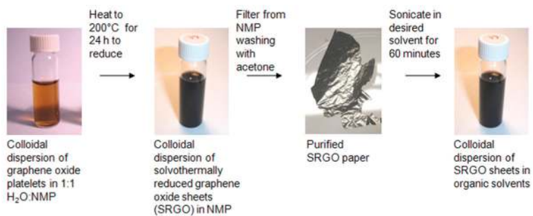
Figure 1. Schematic diagram shows the preparation and purification of solvothermally reduced graphene oxide (SRGO) to create homogeneous colloidal dispersions of SRGO sheets.
