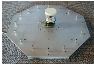
Figure 6: The Panocam Sensor. A video camera and panoramic lens is situated at the centre of a 16-element microphone array. The array is 57 cm in diameter and generates a main lobe which can be dynamically steered along the horizontal plane.
