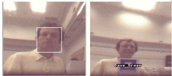
Figure 4: Face (left) and marker (right) detection used to locate potential talkers. The marker allows for talker identification, as does the face detection if the facial recognition system is employed.
