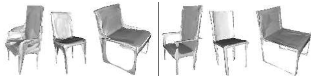
(a) Not trained on chairs (b) Trained on all categories Figure 4. Generalization. (a) Our method (25 patches) can generate surfaces close to a category never seen during training. It, however, has more artifacts than if it has seen the category during training (b), e.g., thin legs and armrests.
