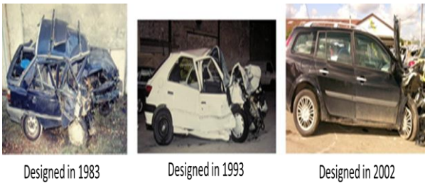
Fig. 1. Evolution of car's in-depth accident analysis (65km/h) – Driver dead, injured and finally intact [6].
