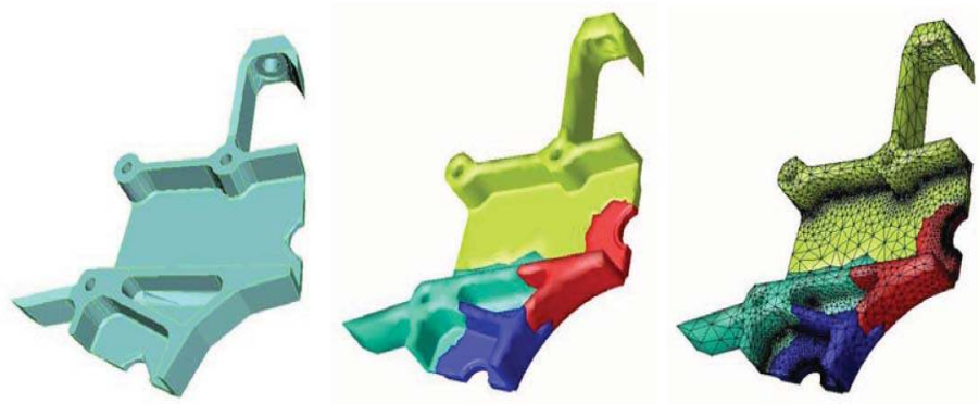
Figure 2.11: Hierarchy of domain decomposition: geometry model, partition model and distributed mesh on 4 processors [24]
