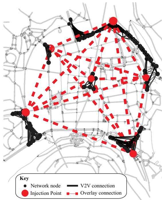
Figure 2: Network with 248 nodes including 6 injections points composing the overlay network in Luxembourg city.
