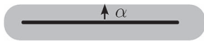
Fig. 2. Buffer operation results in a bounding shape with a width defined by \alpha .
