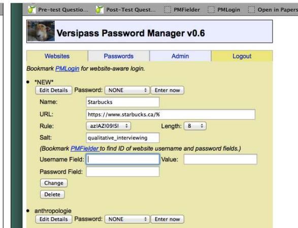
(d) The user chooses a password rule and length from drop-down menus, and inputs a user-chosen salt. The salt can be any string, and does not need to be a secret.
