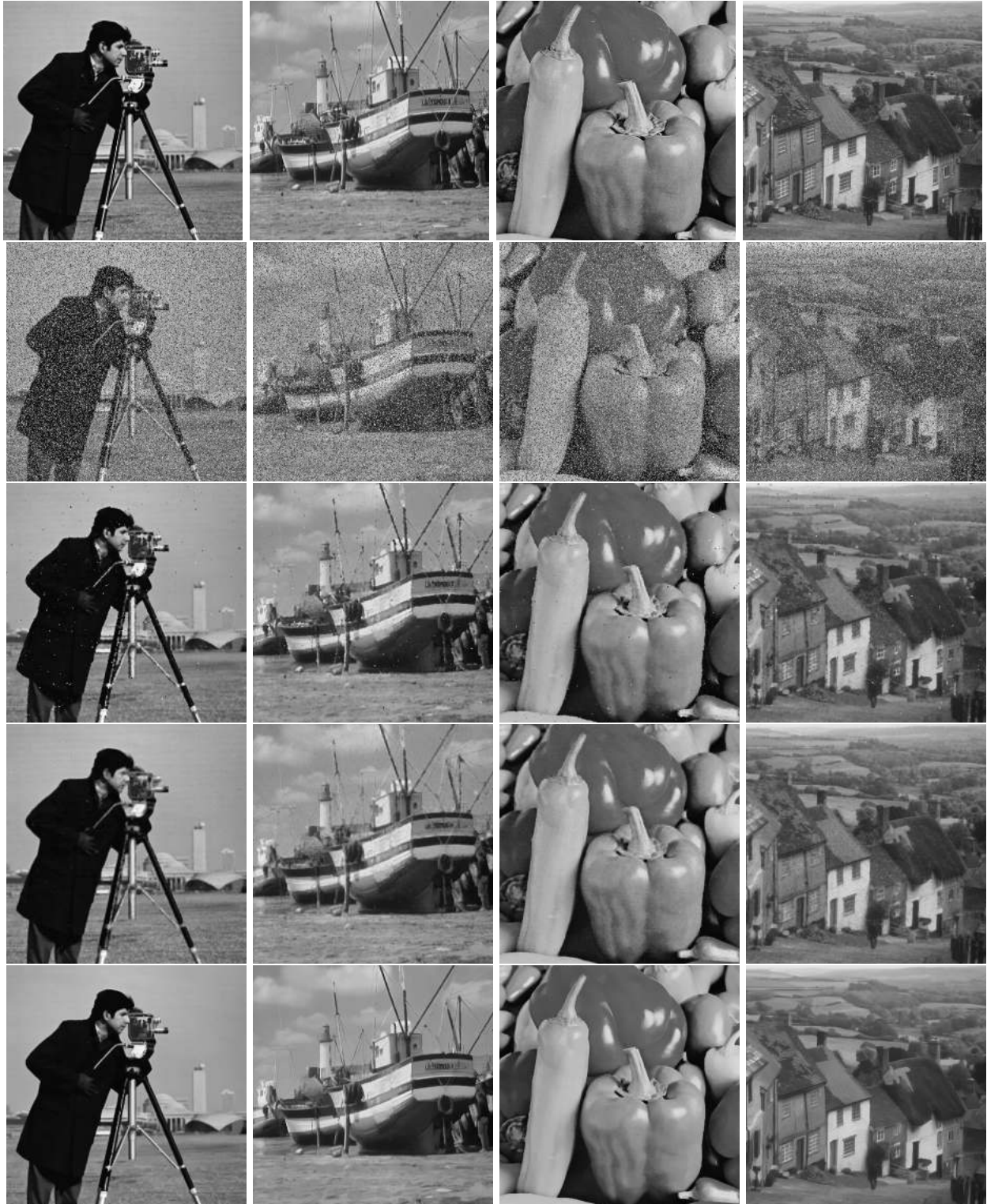
FIG. 6.4. Comparative results on Cameraman , Boat , Peppers and Goldhill with p = 40\% of random-valued impulse noise. For each column, from top to bottom: original image, noisy image, ROAD+trilateral [25], ROLD+EPR [21], PARIGI. Images should be seen at full resolution on the electronic version of the paper.
