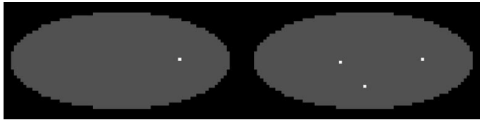
Fig. 2. Simulation objects to compare uniform resolution PL reconstruction to postsmoothed MLEM. Left: the object used to determine the local impulse response. Right: two more points were added for the SNR measurement.
