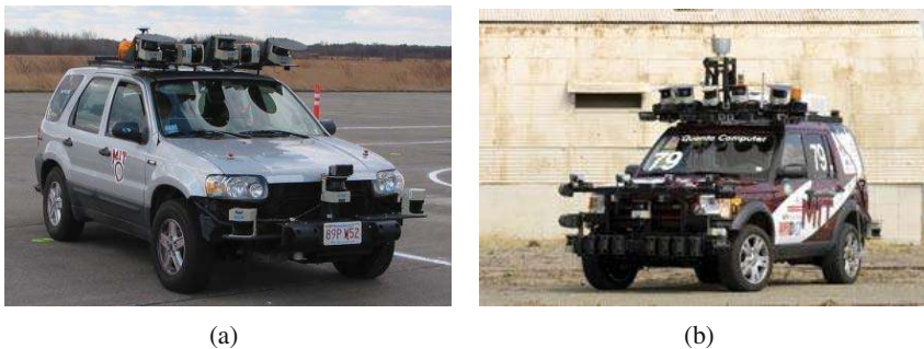
Fig. 3. Developed vehicles. (a) Ford Escape rapid prototype. (b) Talos, our Land Rover LR3 race vehicle featuring five cameras, 15 radars 12 Sick lidars and a Velodyne lidar.
