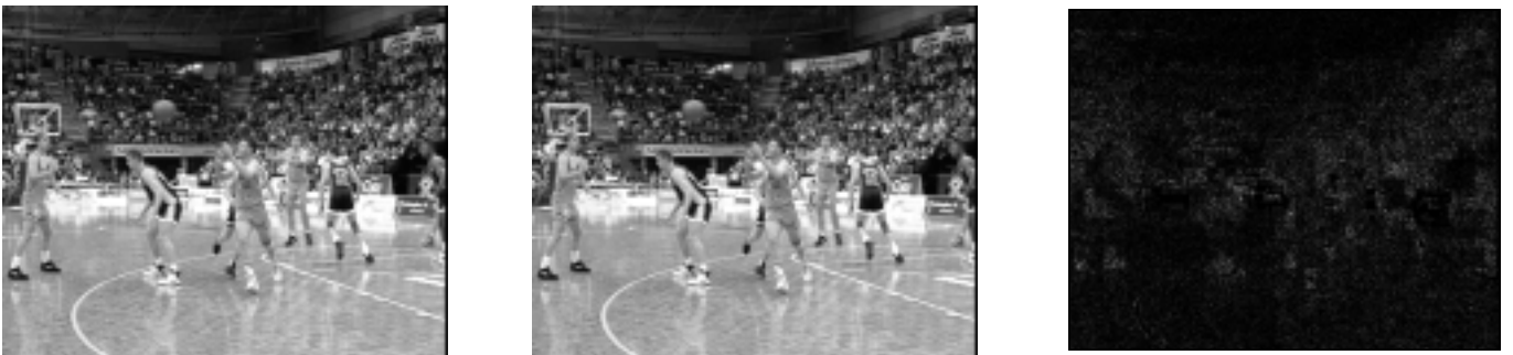
Figure 8. A sample frame from the “Basketball” sequence. The reference, its encoded counterpart, and the pixel-wise difference between them are shown (from left to right).
