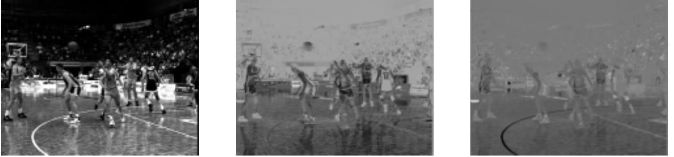
Figure 9. The B-W, R-G and B-Y components resulting from the conversion to opponent-colors space (from left to right).
