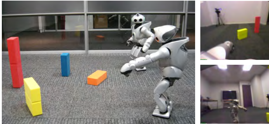
Fig. 5.6 Demonstration of a Sony humanoid robot drawing the attention of the other robot to an object in the shared environment by pointing at it. The images at the right show the scene as seen through the camera of the pointer (top) and the robot observing the pointing (bottom). However, please note that the robots are not able to detect pointing gestures using their built-in cameras. Instead, they directly transmit x, y coordinates of the object pointed at.
