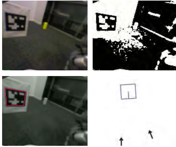
Fig. 5.7 Using objects enhanced with visual markers for estimating the position and orientation of the other robot. Top left: A 2D pattern attached to a carton box as seen through the camera of a Sony humanoid robot. Top right: Binary image generated from the original image. Bottom left: The marker as detected by the ARToolKit tracking system. Bottom right: Both robots send the position and orientation of the carton box (blue) to each other and are thus able to deduce the position and orientation of the respective other robot.
