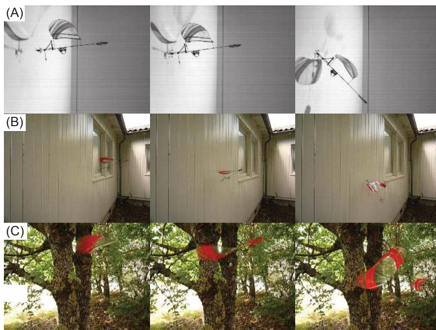
Fig. 11 Perching sequence of the microglider tested to (A) a wallpaper wall, (B) a wooden facade and (C) a Marble tree
