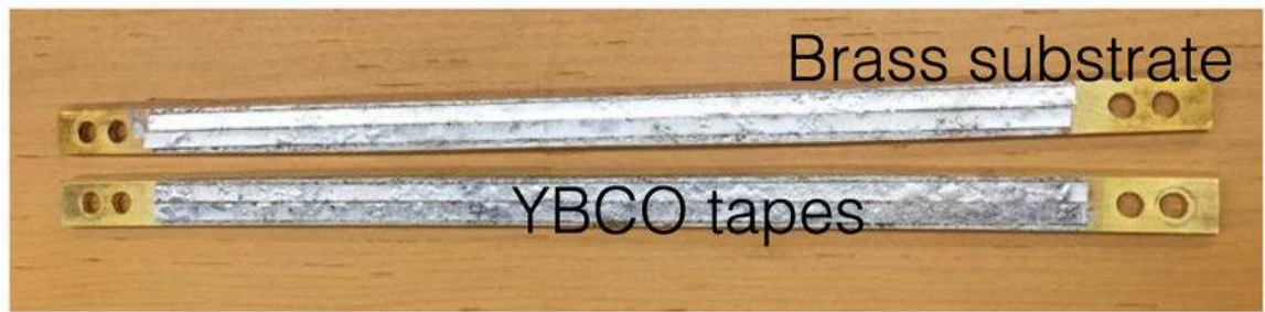
Figure 8. Brass-HTS hybrid leads, YBCO conductors soldered on brass bars.
