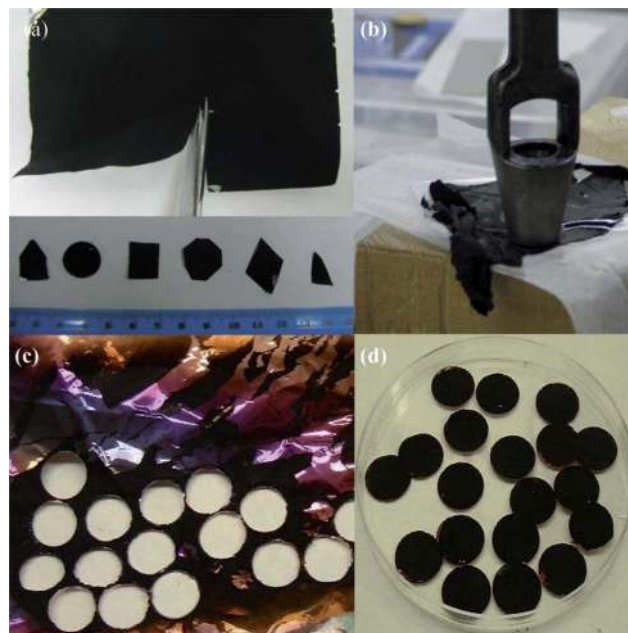
Fig. 3 (a) SWNT macro-film on the metal substrates is cut to various shapes. (b) Free-standing SWNT macro-films. (c and d) Disk electrodes punched by SWNT macro-films on Cu foils.
