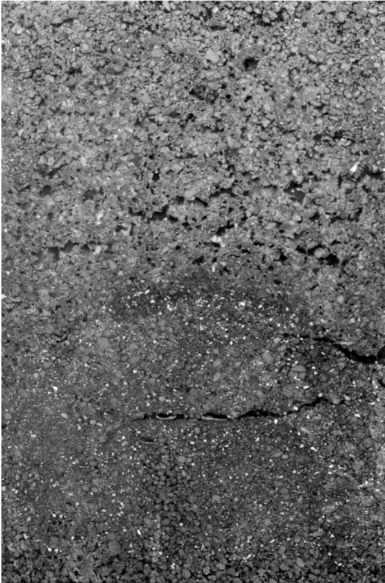
Fig. 10. Quenched sintering bed showing major transformation in bed structure. The flame front was at the middle of the bed.
