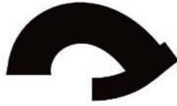
FIGURE 9. Local equilibrium deformation for the mechanical problem in Figure 7 which reverses the orientation of the crossbeam and cannot be reached mechanically starting from the configuration in Figure 7, left.
