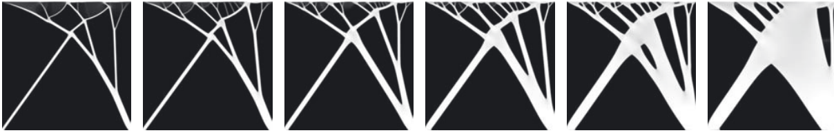
FIGURE 13. Optimal designs with respect to \mathcal{J}_C^\varepsilon for the same load case as in Figure 6 with parameters F = 0.016 \cdot \sqrt{2} , \lambda = \mu = 80 , \eta = 2^k \cdot 10^{-8} , \nu = 2^{5+k} \cdot 10^{-7} for k = 6, \dots, 1 from left to right (resolution 512 \times 512 ). The load is chosen very small so as to stay in the regime of linearized elasticity such that buckling cannot occur for the fine shapes on the left.
