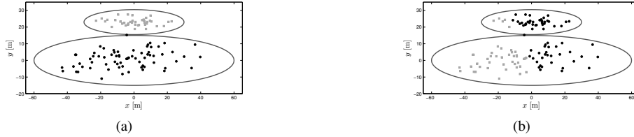
Fig. 2. Illustration of Sub-Partition. (a) Two spatially close extended targets, with corresponding measurements in black and gray. (b) Sub-cells resulting from K -means++, shown in black and gray. Ideally, the measurements should be split into two sub-cells along the y = 15 line.
