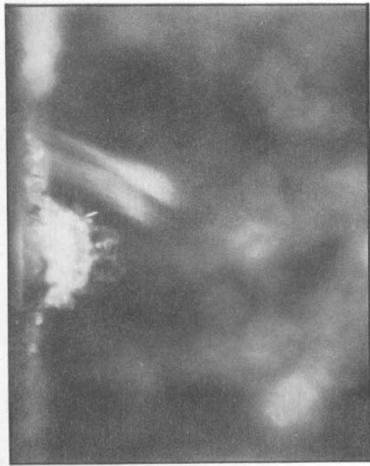
Fig. 17 Photomicrographs of a 1/16 x 1/16 inch specimen of CR-39 after 5 minutes of cavitation damage.
