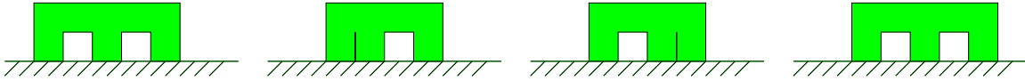
Figure 1: This figure demonstrates using shape metamorphosis for locomotion. A statically stable gait is used to translate the robot from left to right.
