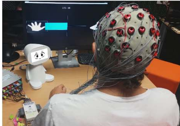
Figure 1: A participant training to use a BCI. He is learning how to perform different MI tasks (imagining a left-hand movement, performing mental calculation tasks and imagining an object rotating) to control the system. Along the training, PEANUT (on the left) provides users with social presence and emotional support, using interventions composed of facial expressions and pronounced sentences adapted to their performance and progression.
