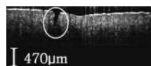
Fig. 3. Optical coherence tomography (OCT) image of a microchannel formed in porcine skin by the microneedle roller. The scale bar indicates a length of 470 \mu\text{m} .
