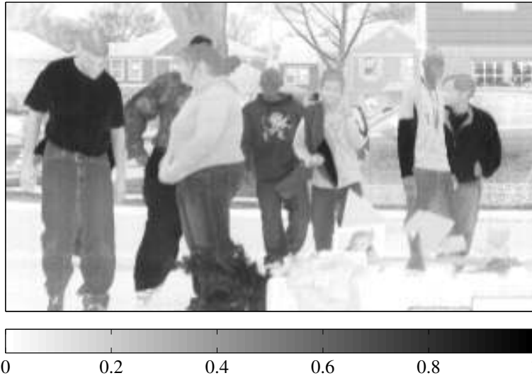
Figure 64: Application of NDVI to the suburban test scene with possible false alarm sources.
