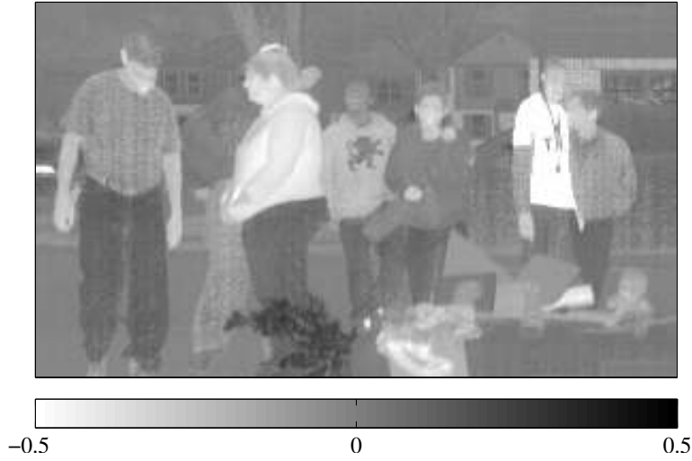
Figure 68: Application of NDGRI to image of suburban test scene with potential skin color confusers. Colorbar shows the representative NDGRI values.
