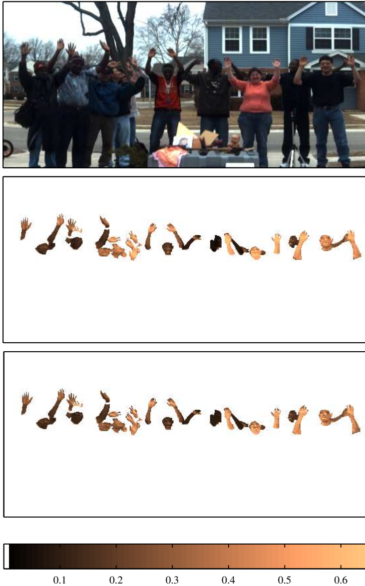
Figure 72: Top: Test scene with seven subjects of interest covering the range of Fitzpatrick skin types. Middle: Skin reflectance at 685nm estimate based on estimated reflectance of skin pixels at \lambda = 685\text{nm} . Bottom: Skin reflectance at 685nm estimate based on estimated reflectance of skin pixels at \lambda = 850\text{nm} .
