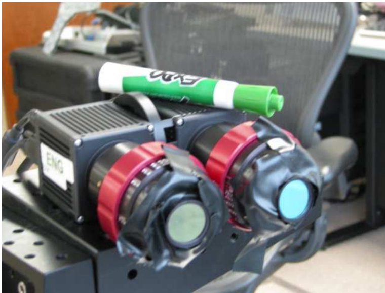
Figure 73: Goodrich near-infrared cameras with optical filters at 1050nm and 1550nm (approximately the specified NDSI wavelengths of 1080nm and 1580nm) with bandwidths of 10nm and 12nm respectively. This demonstrates the flexibility of the methodology developed in this dissertation.
