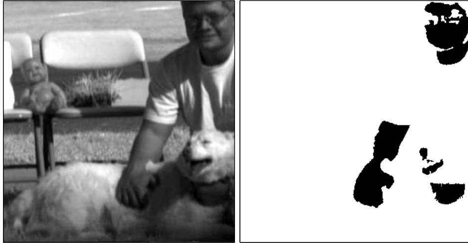
Figure 78: Left: NIR image of a man and his dog. Right: Application of the NDSI thresholded to yield a detection mask.
