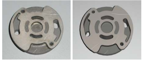
Figure 12: A real scratched metallic part (left) and its corresponding synthetic image (right).
