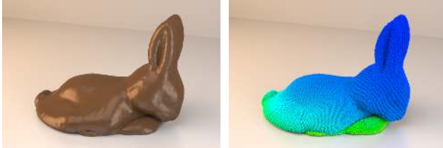
Figure 11: Melting chocolate bunny. Left: Rendered mesh. Right: Particles with color-coded temperatures.
