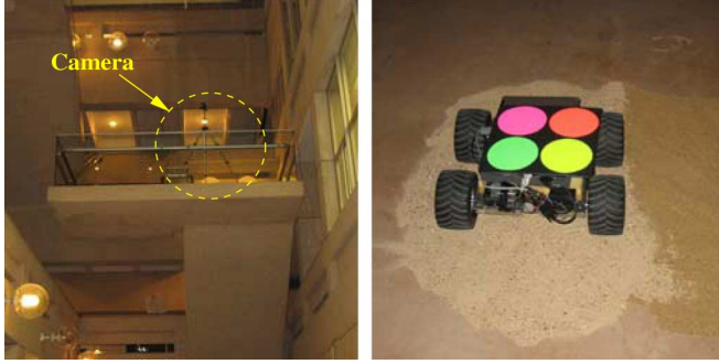
Fig. 9. Computer-vision-based localization system. A high-resolution camera is located at a high location to localize and record the position information of a skid-steered mobile robot.
