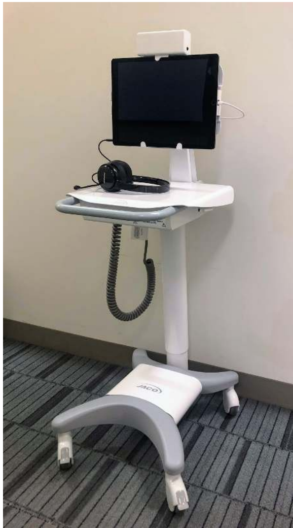
Figure 1. TeleSUDE apparatus consisting of an Apple iPad Pro tablet computer mounted on a locking JACO mobile tablet cart.
