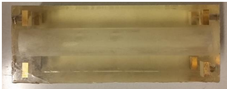
Fig. 2 Rigid walled phantom representing a healthy CCA.
