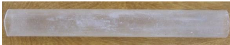
Fig. 1 Thin walled phantom representing a healthy CCA.
