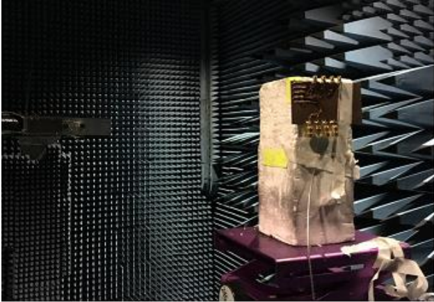
Fig. 17. Measurement setup for the radiation patterns.
