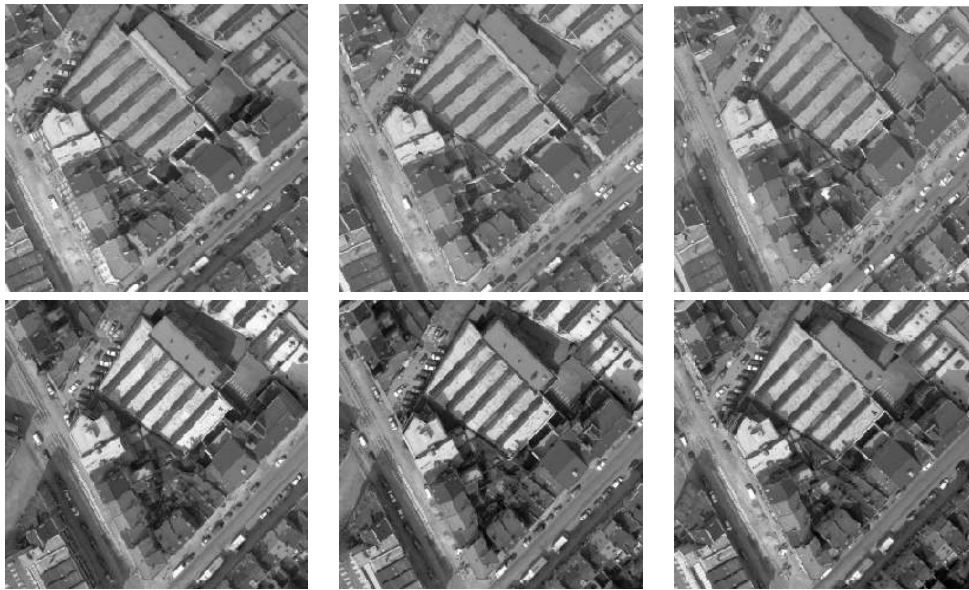
Figure 19: Six overlapping aerial views. The images are about 1200 \times 1200 pixels, one pixel corresponding to a ground length of 8.5cm. The images are acquired at a height of 1300m in two triplets: the camera approximately translated by about 300m between successive views in images 1-3, and between images 4-6. The first set acquired on the outward flight, and the second set on the approximately parallel return flight.
