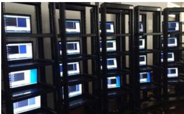
Fig. 14 Distributed simulation hardware platform
