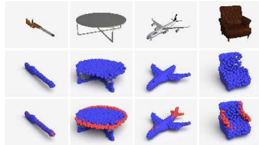
Figure 10. Visualization of points predicted by the deconvolution branch (blue) versus the fully connected branch (red).
