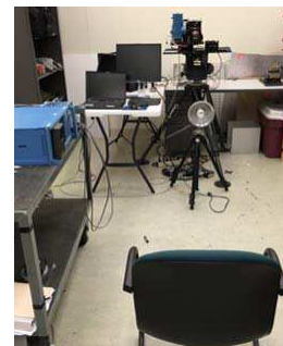
Figure 3: Data collection setup showing the floor lamp and chair at Range 1 (2.5 m). In addition, a cardboard background was placed 0.1 m behind the chair.
